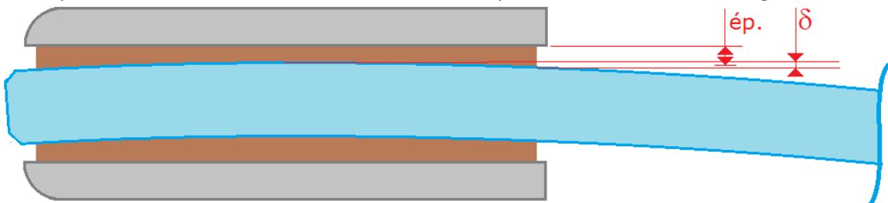
$$\delta \text{ (mm)} \cong \frac{400}{R \text{ (mm)}} \ll 1 \text{ mm}$$
